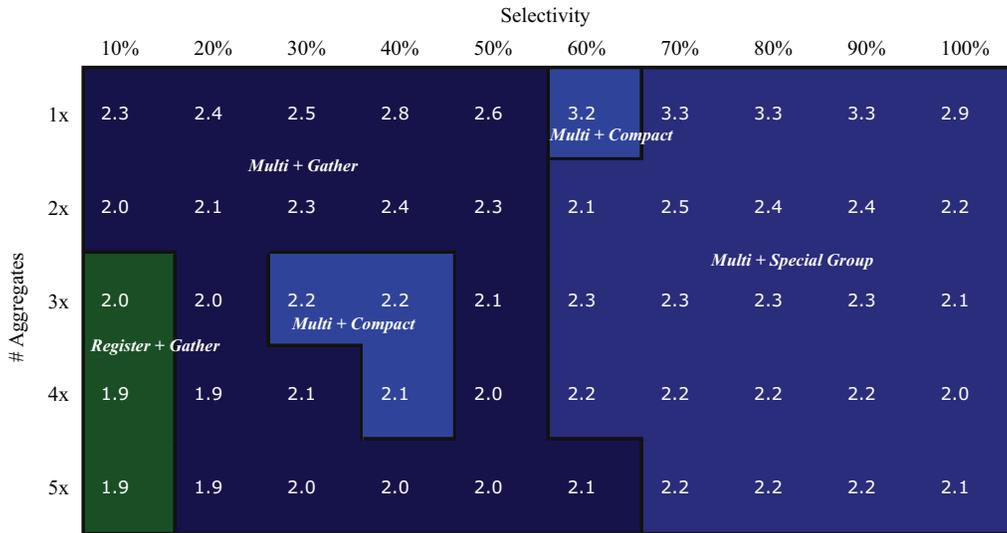
Figure 10: Performance of aggregation techniques, 32 groups, 28 bits encoding
