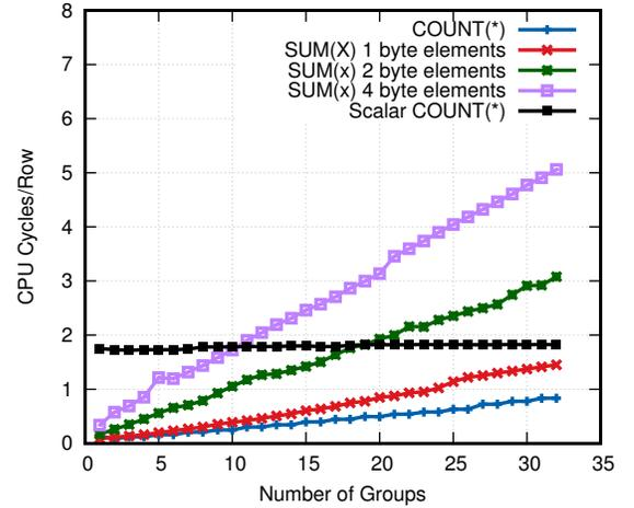
**Figure 5: Performance of In-Register Aggregation**
