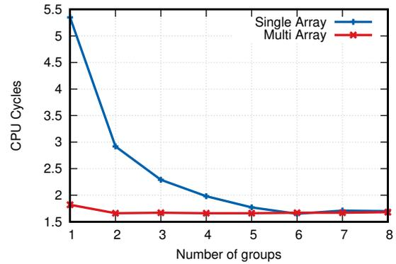
Figure 2: CPU cycles per row for COUNT aggregation
